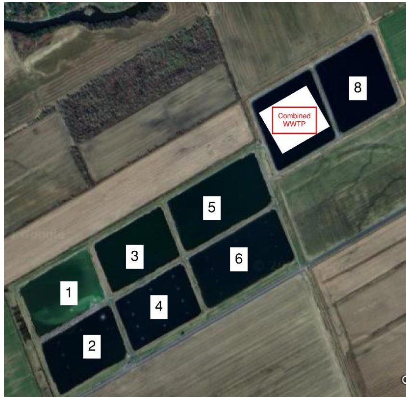
Figure 7-22: Possible Combined WWTP Footprint
