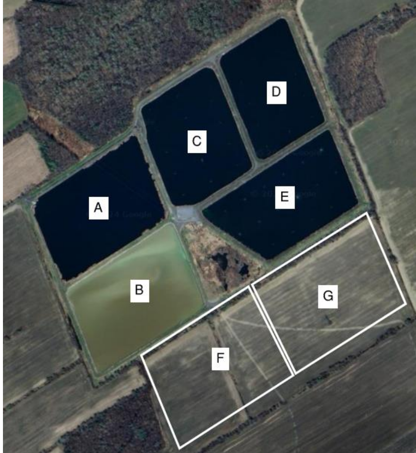
Figure 7-8: Russell WWTP Lagoon Expansion for 2046 Flowrates
