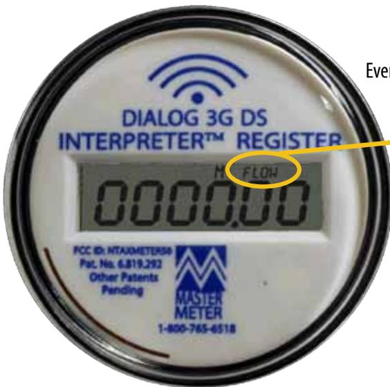
**IMAGE 2 :** Rate of Flow in Meter/minute
